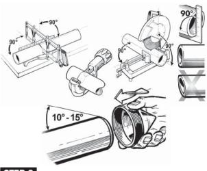
STEP 2 Measure from pipe stop to the end of the coupling.
