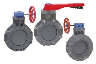
Spears® innovative design departs from traditional liner-seat type valves to eliminate seat creep, reduce operating torque and provide positive seal off. Ideally suited for flow control or throttling, this high performance valve is offered with a full variety of options for greater application versatility. Standard valves are produced from PVC or high temperature CPVC in IPS sizes 1-1/2" through 16". PVC and CPVC True Lug valves are produced in sizes 1-1/2" through 12".
