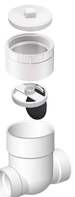
A Backwater Valve is designed to function as a check valve in a drainage pipe to prevent flowing liquid, such as sewage, from reversing its direction. There are other applications for Backwater Valves, such as multi-level pond balancing for Aquascape applications or for storage tank balancing for industrial and agricultural applications. Backwater Valves should not be confused with Backflow Preventers which are used in potable water supply systems.
