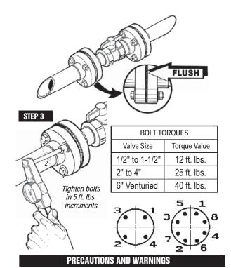
*CAUTION:* The system must be designed and installed so as not to pull the components in any direction. Pipe system must be cut and installed in such a manner as to avoid all stress loads associated with bending, pulling, or shifting. All piping systems must be supported.
