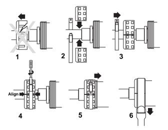
Split Nut Kits are designed to replace broken union nuts on Spears<sup>®</sup> True Union 2000 Ball Valves and Union 2000 Schedule 80 Unions. Can also be used if nut was not in place during end connector installation. Kit includes SS316 Gear Clamp and 2-Split Nut halves. Install Split Nut Kit as illustrated. Caution: System must be depressurized and drained prior to repairs.
