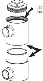
Cap uses O-ring seal, no thread sealant required.
